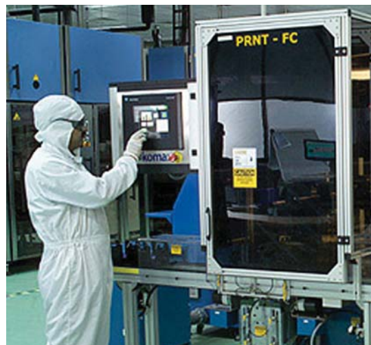
State-of-the-art screen printing technology used in the manufacture of solar cells
